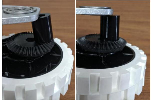
**Step 7a:** Slide the hex shaft the rest of the way through.
