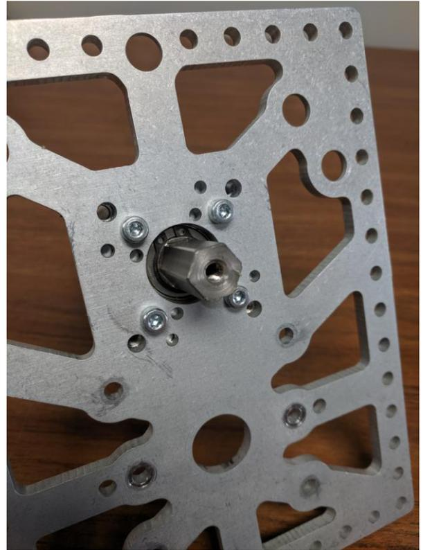
**Step 3c:** Slip the 1/2 in. long 1/2 in. hex spacer (am-3948-500) over the hex shaft.
