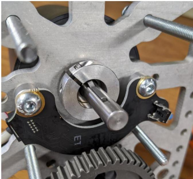
**Step 12d:** Place the 4 long aluminum spacers on the protruding BHCSs from step 5d
