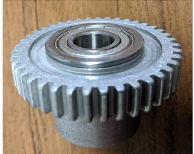
**Step 4b:** Press the gear/bearing assembly from Step 2b into the large bearing. Note the orientation of both parts in the pictures.
