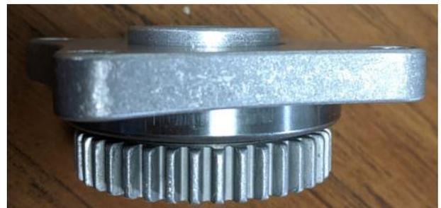
**Step 5b:** Place the large washers (am-1534) and thrust bearing (am-1535) in a sandwich on the protruding part of the bearing gear.
