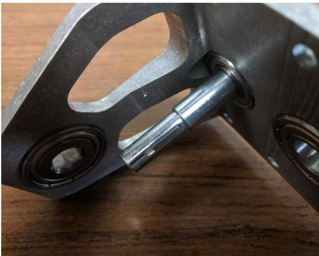
**Step 4a:** Install the 8mm bore bevel gear (am-2621) onto the shaft and secure in place with a push on retaining ring (am-0033).
