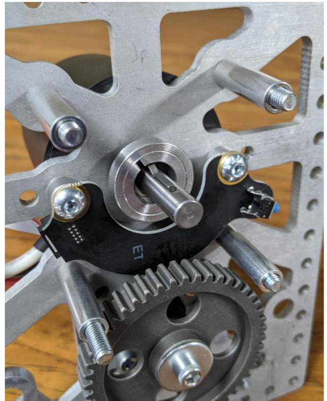
**Step 13d:** If using a CIM or NEO align the slot in the drive shaft with the keys in the motor shaft and press the motor shaft into the drive shaft.
