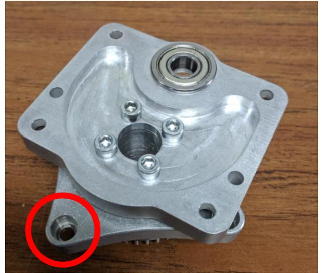
**Step 7b:** (Optional) If you are using a Lamprey encoder apply a few drops of super glue to the ring around the 1/2 in. bearing. Press the magnet down onto the glue and give it approximately a quarter turn to disperse the glue. Hold for 30 second while the glue sets.
