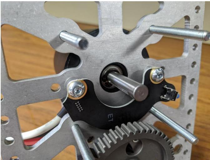
**Step 8d:** (Optional) If using the Lamprey encoder, insert the ribbon cable in the orientation shown.
