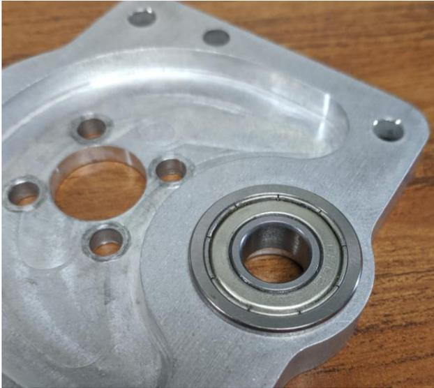
**Step 2b:** Press the 1/2" round bearing (am-0030) into the bearing gear (am-3013b)
