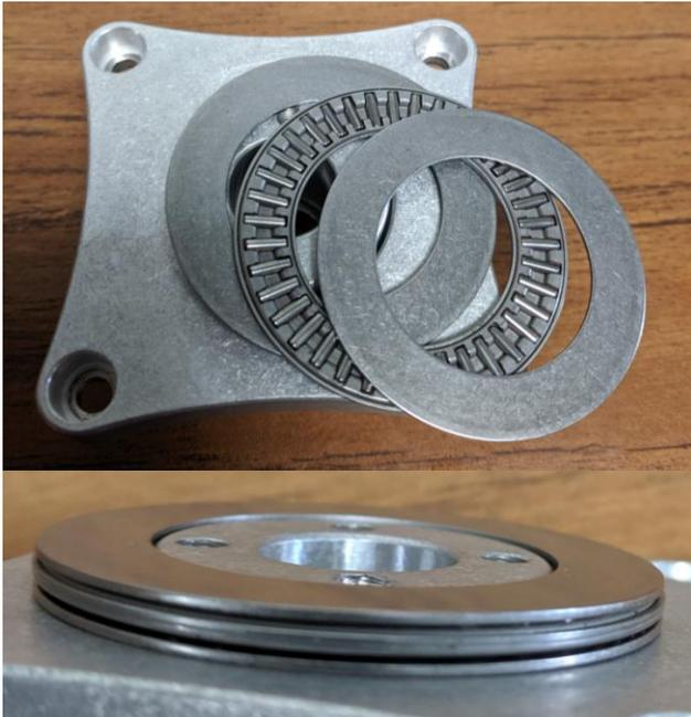
**Step 6b:** Screw the gear plate with bearing from Step 1b to into the tapped holes on the gear from Step 2b using (4) 10-32 screws with thread locking patch (am-1120). This completes am-3009\_center.
